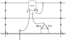
*Note:* If required, this energizer can be used as part of a solar installation, by connecting it to a battery and solar panel(s). For information about solar installations, refer to the product's website (see packaging for details).
