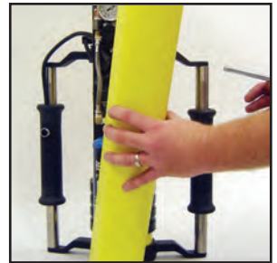
C. Pull ball lock pin and remove cover.
