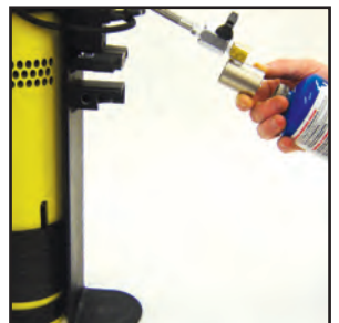
E. Carefully unscrew tank from the tank adapter.
