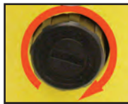
Turn knob clockwise to increase pressure.
