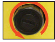
Turn knob counter clockwise to decrease pressure.
