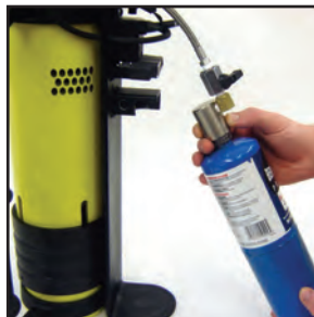
D. Remove tank from the tank mounting bracket.
